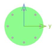
DefinitionReinforcementMaterialConcreteTypeDescriptionPosition(s)Grade5000 psiCIRCLE8"Grade 60"28.70,0 210ProfileSTD C 508
