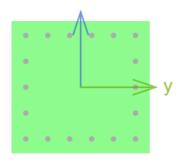
DefinitionReinforcementMaterialConcreteTypeDescriptionGradeC30/37PERIMETER18A25ProfileSTD R 620 650
