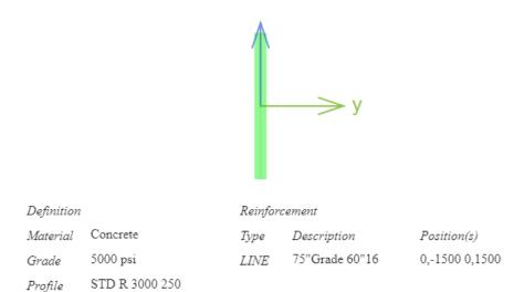
When: analysed for an axial load equal to its ultimate axial load capacity (compression) of -4244800.000000kN
