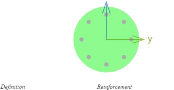
MaterialConcreteTypeDescriptionPosition(s)Grade4750 psi user definedCIRCLE8"Grade 60"320,0 192ProfileSTD C 508
