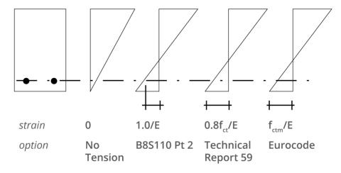
Integrating the stresses from this strain plane over the section will give an axial force equal to the applied force, and a moment which is parallel to the applied moment. The value of this moment is the cracking moment. Short-term material properties are always used for the cracking moment calculation.
