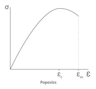
These have been adjusted and are based on the Thorenfeldt base curve.
