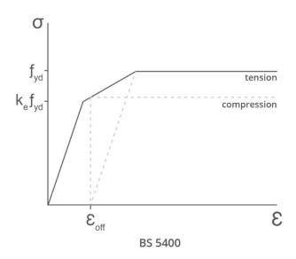
In tension the initial slope is defined by the elastic modulus, E, until the stress reaches  $k_e f_{yd}$ . The slope then reduces until the material is fully plastic,  $f_{yd}$ , at  $\varepsilon = \varepsilon_{off} + f_{yd}/E$ . Post-yield the stress remains constant until the failure strain,  $\varepsilon_u$ , is reached. For BS5400  $k_e = 0.8$  and  $\varepsilon_{off} = 0.002$ .
