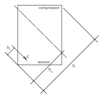
where c is the centroid of reinforcement in tension. The strain term is given in the code as
