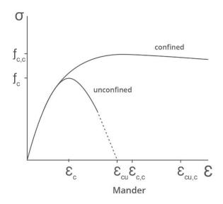
For unconfined concrete, the peak of the stress-strain curve occurs at a stress equal to the unconfined cylinder strength  $f_c$  and strain  $\varepsilon_c$  generally taken to be 0.002. Curve constants are calculated from
