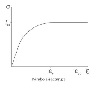
If the curve is taken to be tangent to the plateau then at  $\eta=1$ , f'=1 and  $\frac{df'}{d\eta}=0$
