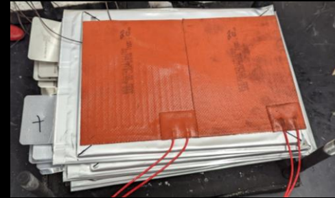
Top cell covered by heat pad and temperature sensor in between
